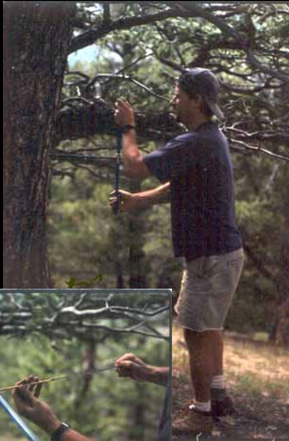
An increment borer is used to sample cores from about 20 trees at a site
