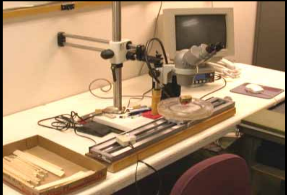
Cores mounted and sanded, then dated, measured, and averaged into site tree-ring chronologies
