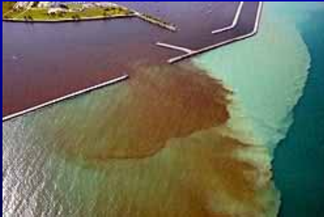
Combined Sewer Overflow (CSO) Plume in Lake Michigan (Milwaukee Harbor).
