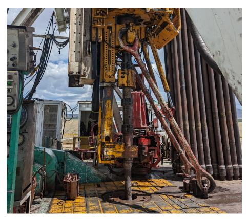
The drill at Utah FORGE, where they are currently in the process of drilling a 10,000-foot-deep geothermal well to test Enhanced Geothermal Systems.
